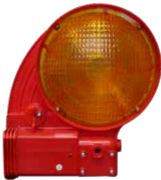
Signal light for traffic panels PowerNox with radio frequency for connection in series with integrated transmitter and built-in antenna (receiver) for mounting on safety traffic panels and panel fences, with LED technology, constant flashing light, one-sided yellow optics Ø 180 mm with dusk-to-dawn function approved for highways and all other streets, with lateral battery box BAST tested
